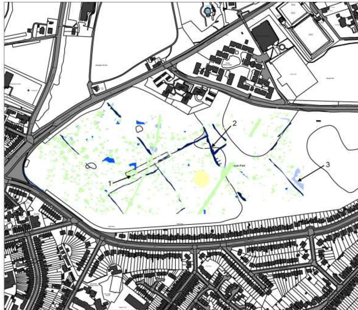
Figure 8: Interpretation of gradiometer survey results
