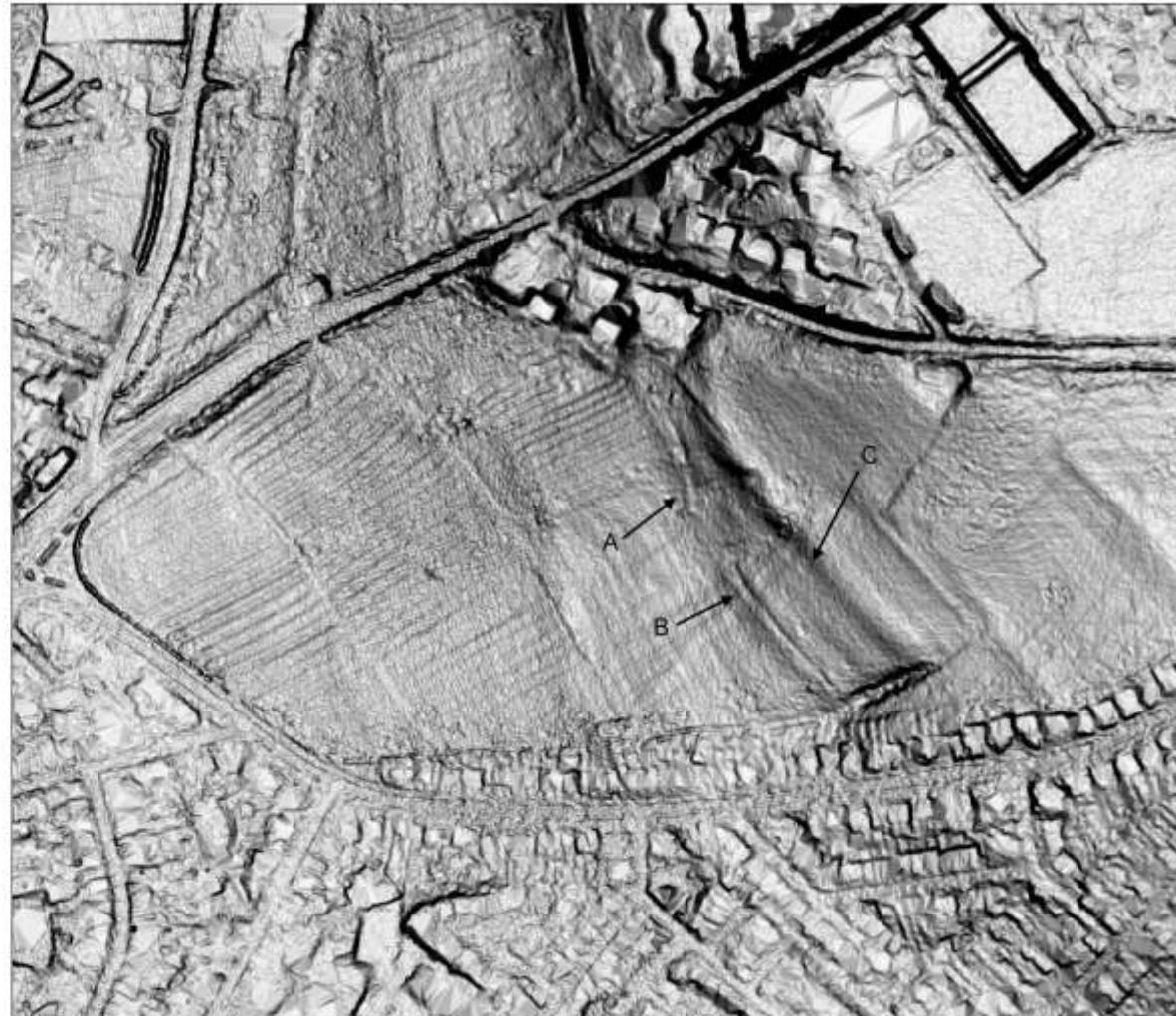
Figure 14: Slope model (darkest = steepest) derived from 1m LiDAR DTM
