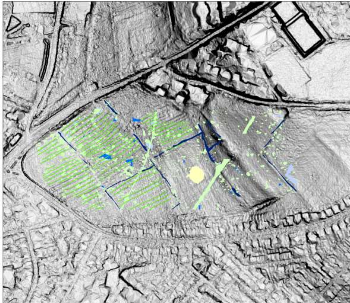
Figure 15: Slope model (darkest = steepest) derived from 1m LiDAR DTM and gradiometer survey results
