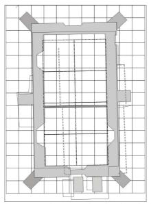
Fig. 3 Structural masonry and mortar at the east end of the chapel (shaded) (drawn by the author)
