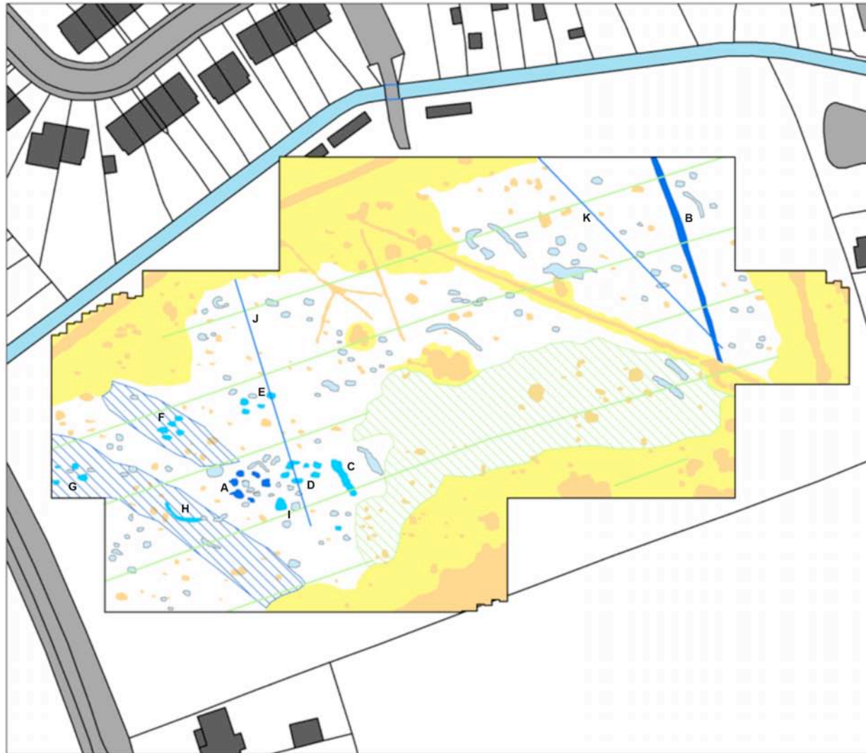
Figure 11. Interpretation of real time gradiometer survey data
